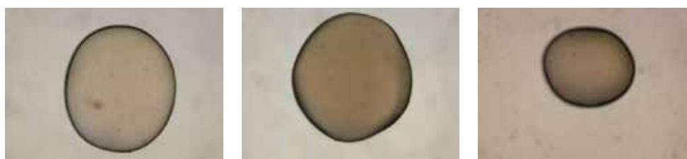
Fig. 5.7. The beads prepared from 80% PRC, 55% PRC and 30 % PRC respectively
